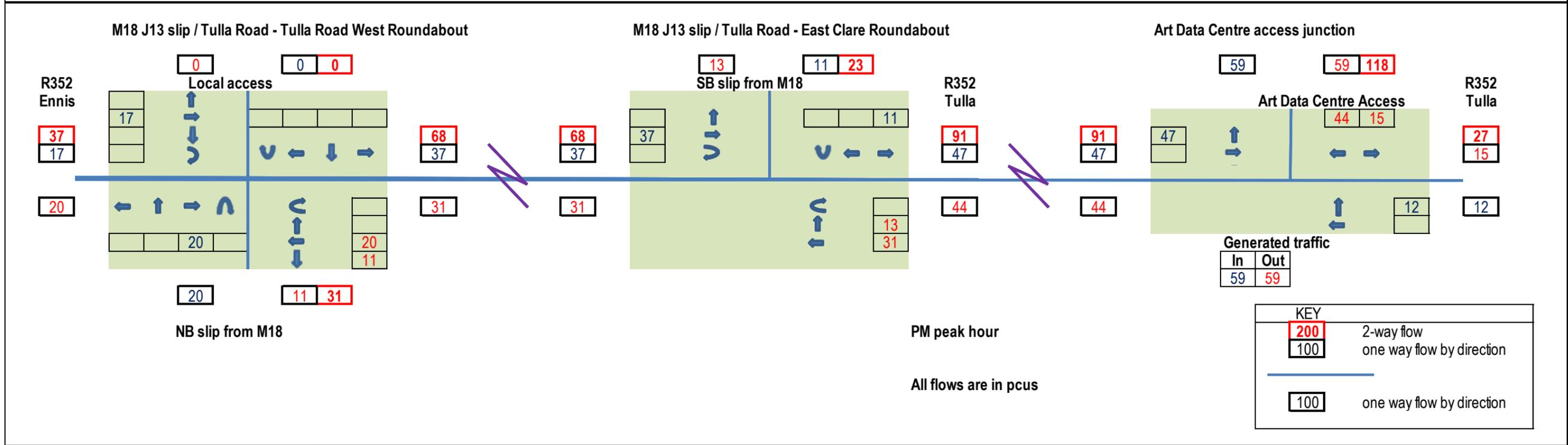
Figure A12.3.18 Generated total trips, weekday AM and PM peak hours - Art Data Centre fully operational, all vehicles - pcus
