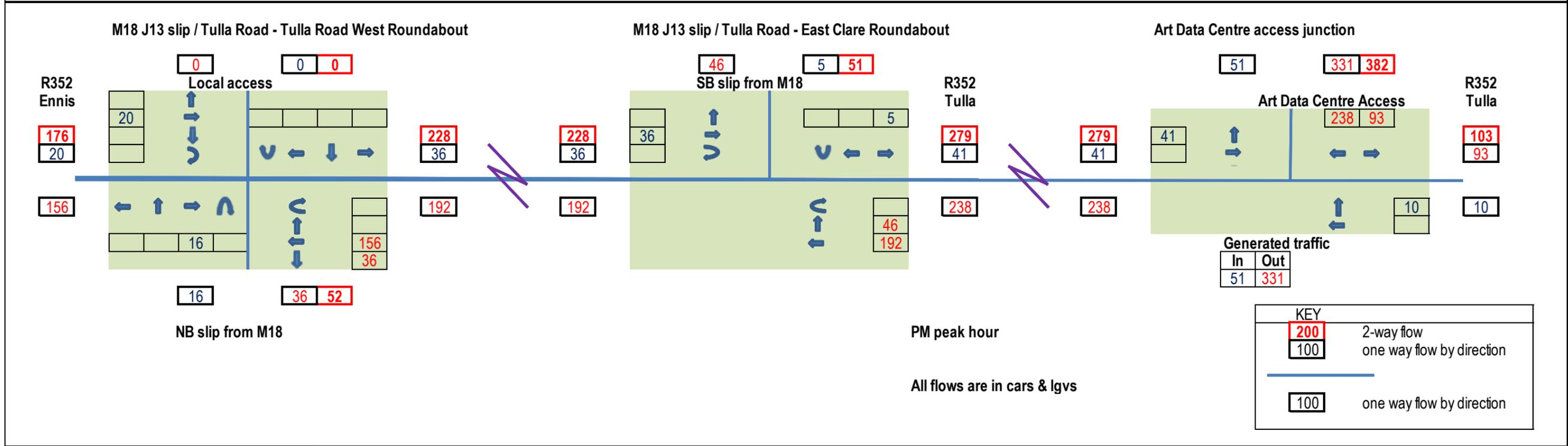
Figure A12.3.11 Generated car/ligv trips, weekday AM and PM peak hours - Art Data Centre peak construction, year 2027 - cars/ligvs
